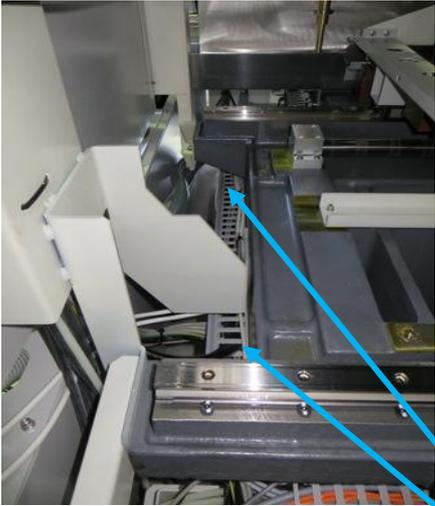
cable guides between machine and tank
