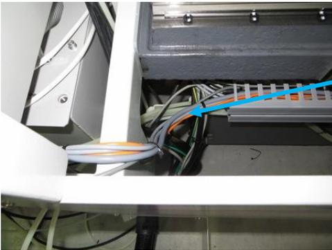
Wire the cables from the PCNC to the safety-box. Fix the cables with ties.
