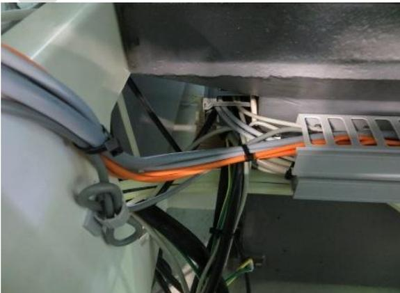
Wire the sensor-cable to the safety box
