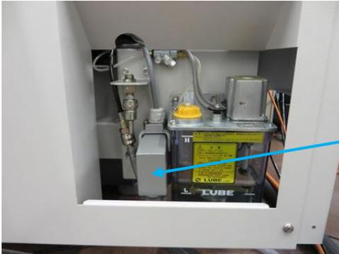
Harting connector on MP2400 (back side of machine)
