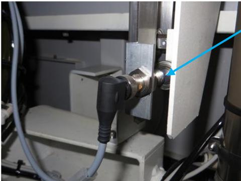
opened front door , the ball bearing is the conductor for the proximity sensor
