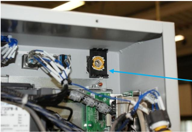
Mount the new mounting latch for the contact-blocks of the emergency switch
