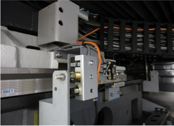
Wire the sensor-cable to the safety box
